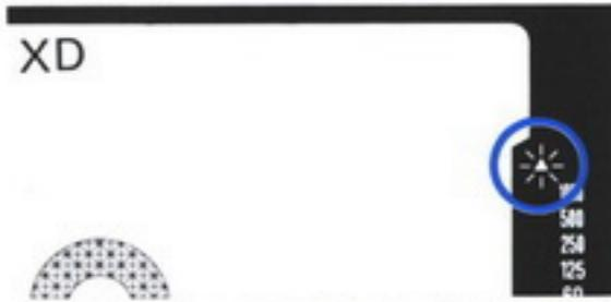
When the Auto Electroflash 118X used with a Minolta X-300, X-370, XD, XG or 110 Zoom Mark II camera, a flash-ready signal in the camera's viewfinder will blink to indicate that the flash has recycled. After it flashes the 118X will switch the camera back to the previously set mode until it has recycled and the signal starts to blink again.
