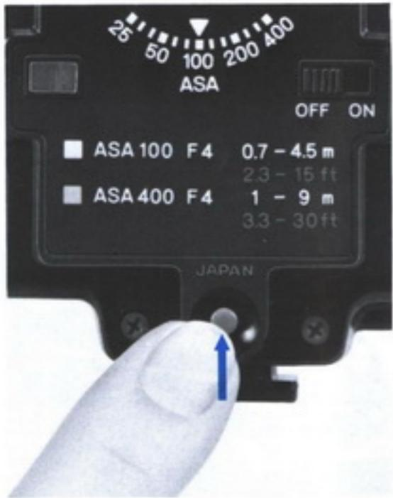
Non-synchronized "open-flash" pictures can be made by disconnecting the camera and flashgun and using them separately. In this case the flash is triggered by pushing the open-flash/test button. Since flash duration is still controlled by the sensor in automatic operation and remains fixed at maximum power on manual, exposure produced will be as indicated in those respective sections.
