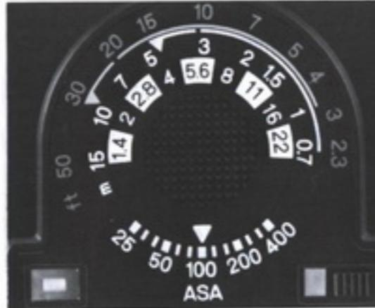
3. For proper exposure with normal subjects and condition, set the lens aperture on the camera to the f-number that appears opposite the flash-to-subject distance on the computer dial (e.g., with a film-speed of ASA 100 or DIN 21 set, the aperture would be f/2 for 9m or 30 ft, f/4 for 4m or 13 ft., or f/5.6 for 3m or 10 ft.)
