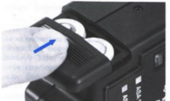
3. Close the chamber by aligning the cover carefully, depressing ends of batteries slightly with it, and sliding it toward the top of the unit until it snaps securely in place.
