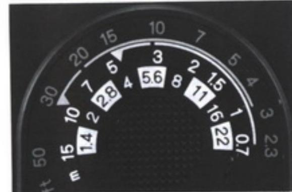
The points on the distance scale opposite the red or yellow auto-aperture/range-indicator arrows indicate the maximum distances for correct auto exposure; subjects farther than these distances will normally be underexposed. Minimum subject distance for the red setting is 1m (3.3 ft.) and for the yellow setting is 0.7m (2.3 ft.), subject distances closer than this will normally result in uneven flash coverage and/or overexposure.
