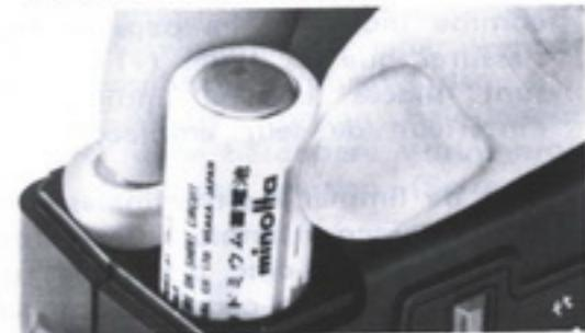
2. After wiping terminals with a clean, dry cloth, insert two carbon-zinc, alkaline or Ni-Cd batteries as specified on p. 43, making sure that plus (+) and minus (-) ends are positioned as indicated inside the chamber.
