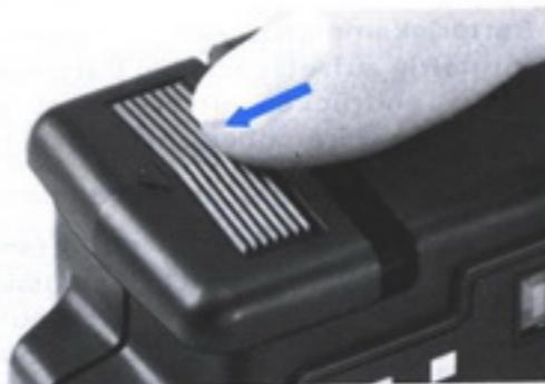
1. Remove the battery-chamber cover by sliding it off in the direction of the arrow toward the bottom of the unit.
