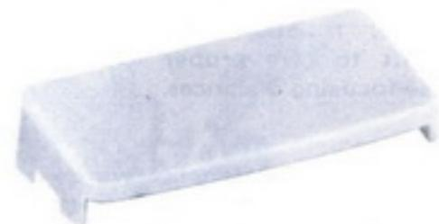
Designed specifically for the 110 Zoom Mark II owner who desires to use a flash for macro photography. This accessory panel clips onto the 118X Auto Electroflash, and directs the light from the flash downward to give precise flash coverage of the subject. It also reduces the flash output to give proper exposure at close-focusing distances.
