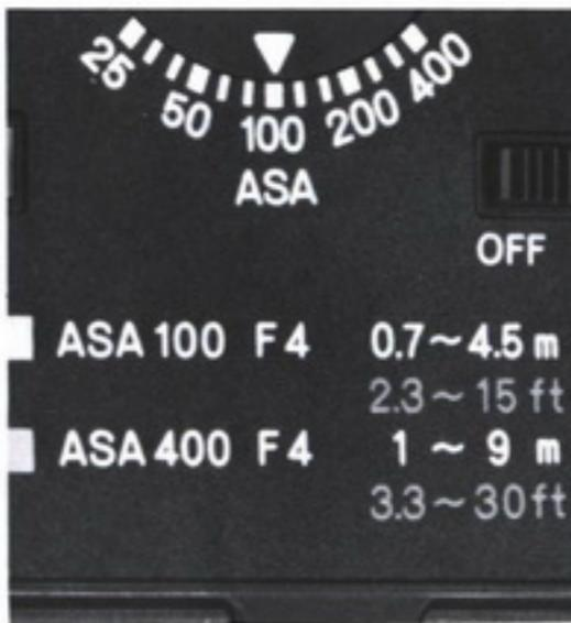
When using ASA 400 or ASA 100 film, you can confirm the autoflash aperture, mode setting and minimum and maximum subject distance for the correct exposure by consulting
