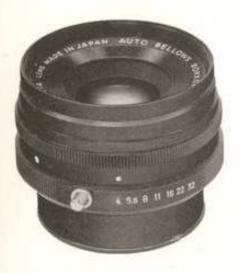
This lens is designed for use with the Auto Bellows I. (See page 34.) It comes in a short mount so that a large enlargement ratio from a greater distance can be achieved, and so that there is greater freedom for the placement of lighting equipment. Focusing range is from infinity (with bellows) to 1:1 image size (lifesize) on the negative. As with other Rokkor Lenses, the 100mm Bellows Lens has a depth-of-field preview button.
